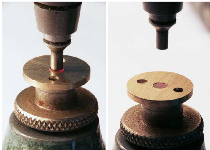
3. Pressing in the endstone 4. The endstone fitted
